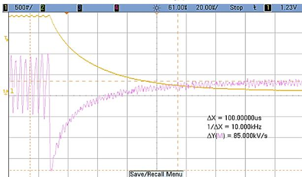
Figure 7. Discharge cycle of the output capacitor
